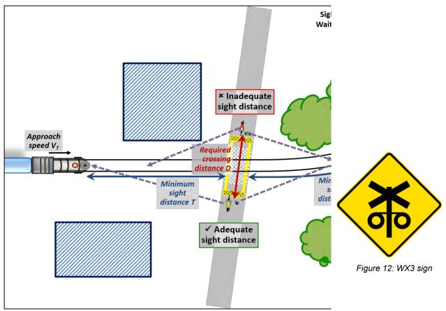
Figure 11: Examples of adequate and inadequate starting sight distance
