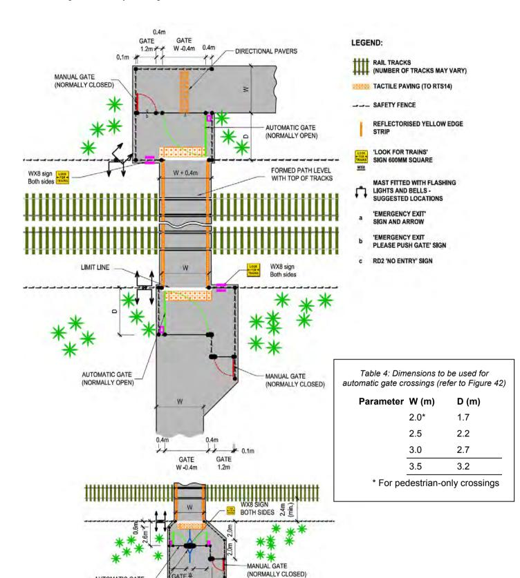
Figure 42: Layout plan for automatic gate crossing
