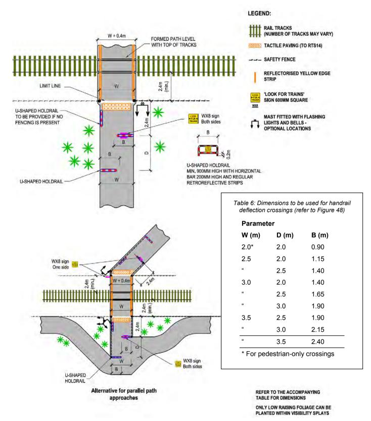
Figure 48: Layout plans for a handrail deflection approach
