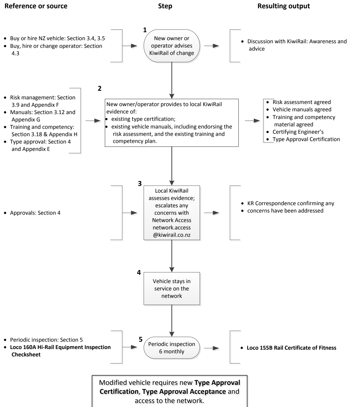
Figure 2: Process for vehicle already approved in New Zealand: changing ownership, changing operator, or hiring vehicle.
