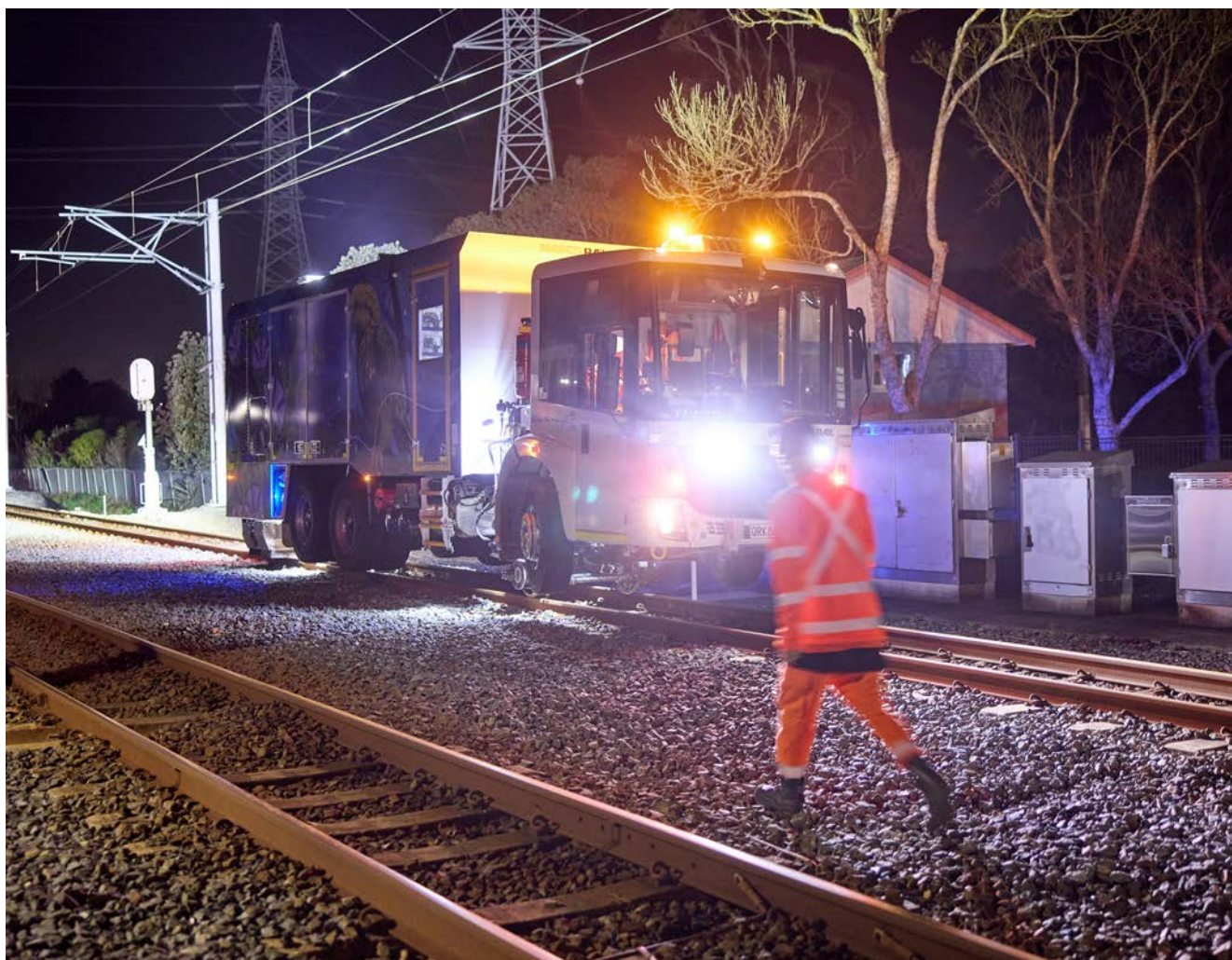
KiwiRail's cutting-edge Automated Track Inspection System (ATIS) enhances track maintenance and safety through advanced diagnostics and measurements on the Auckland metro network
