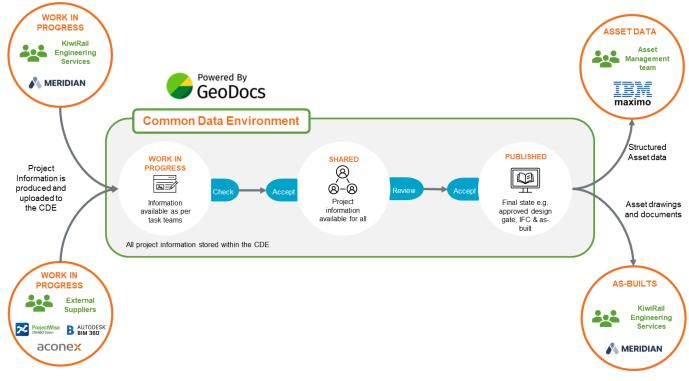
Figure 8: Project Information workflow through KiwiRail Systems
