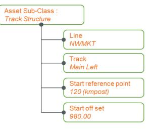
Figure 12: Linear Reference example
