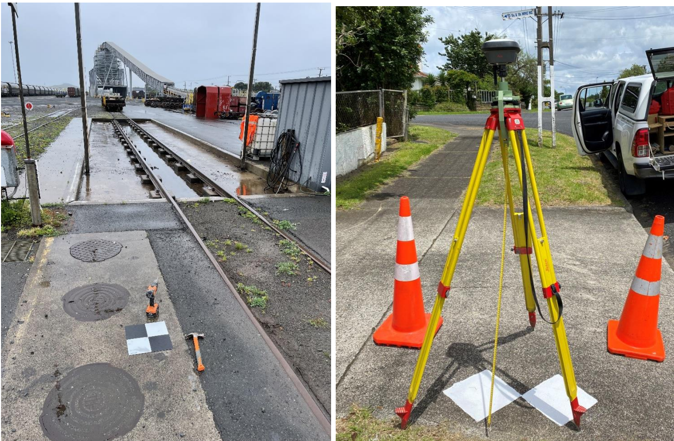
Figure 2: Typical KiwiRail Primary Survey ground control points, marked for identification in aerial photogrammetry
