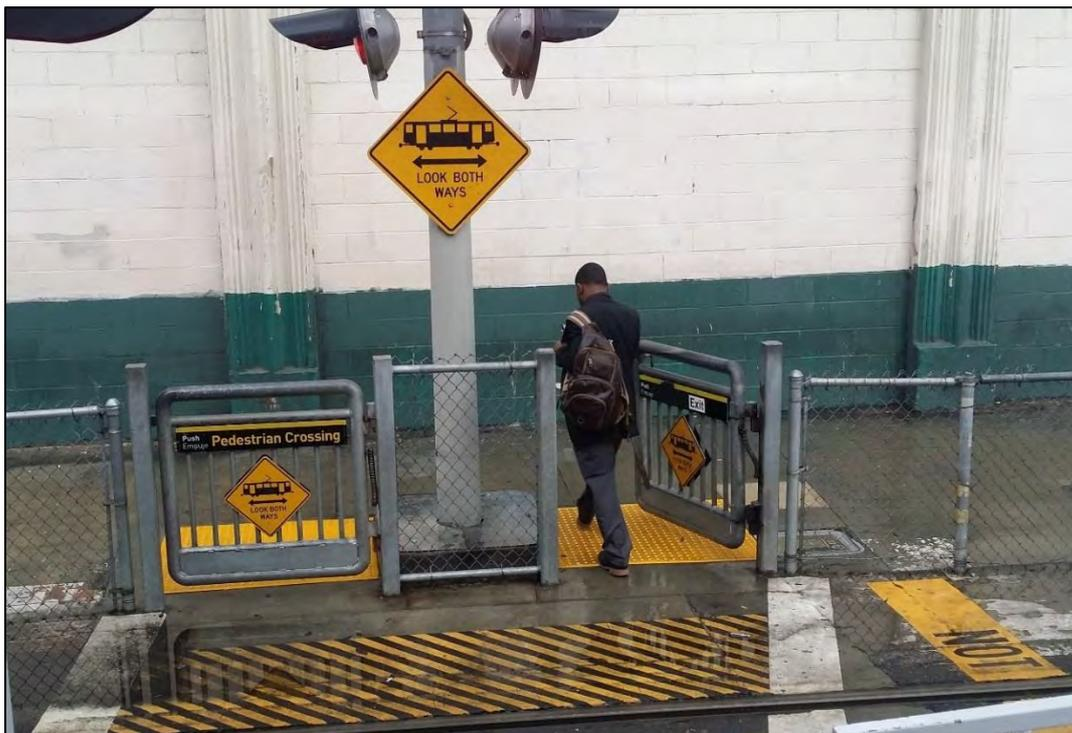
Figure 50: Spring-restrained manual swing gates in Los Angeles (US)
