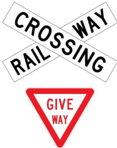
Figure 21: RPX3 level crossing GIVE WAY sign assembly
