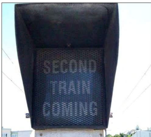
Figure 30: Example of an active warning sign
