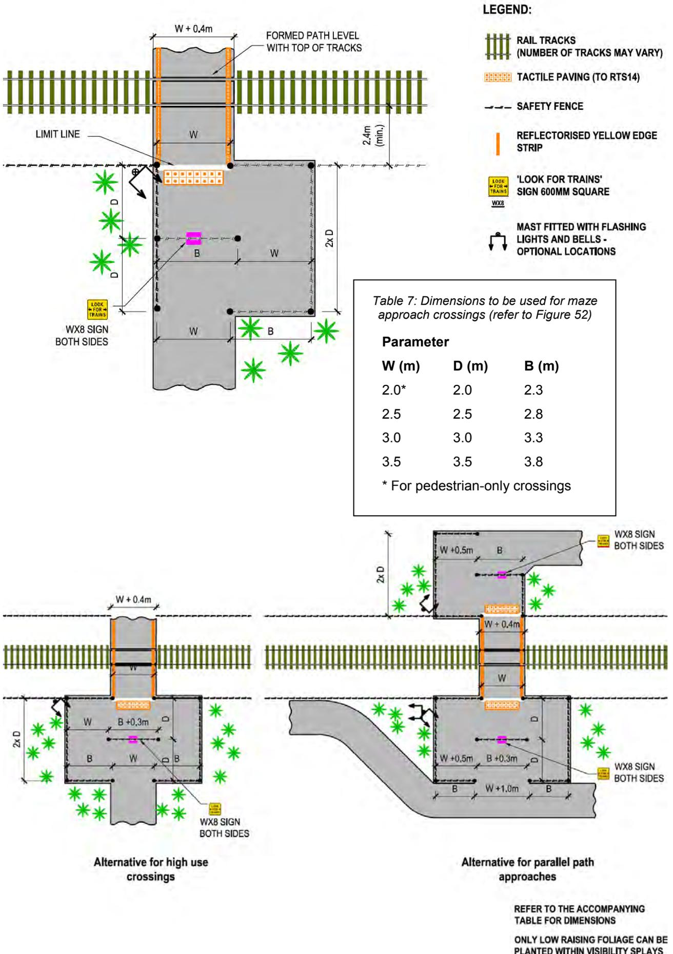
Figure 52: Layout plans for maze approaches
