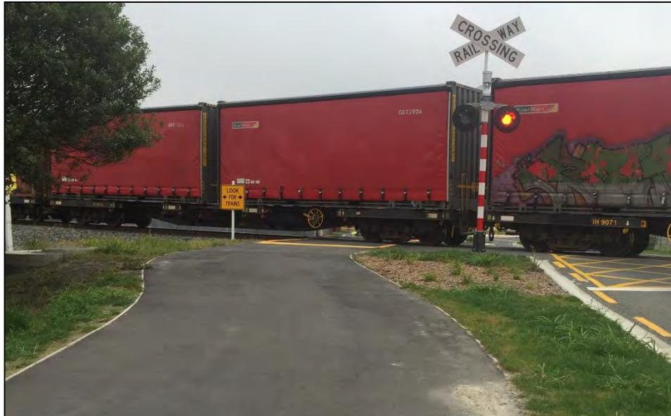
Figure 43: Flashing lights and bells on a path approach (Kaiapoi)
