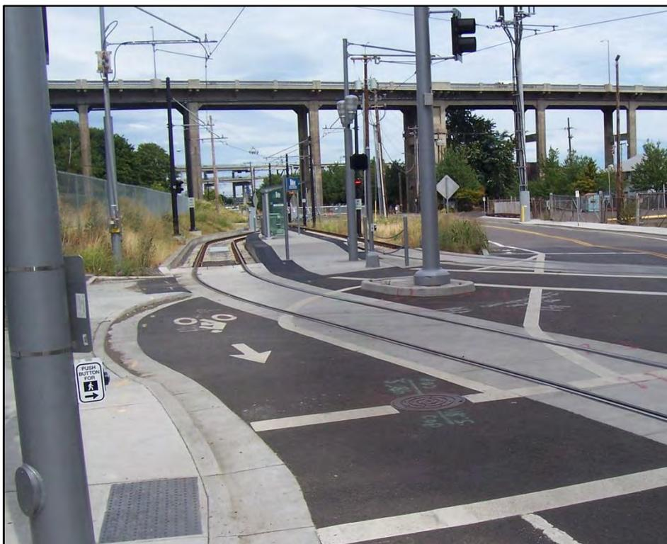
Figure 14: A cycle lane is re-aligned to cross a railway closer to 90 degrees (Portland, OR, US)
