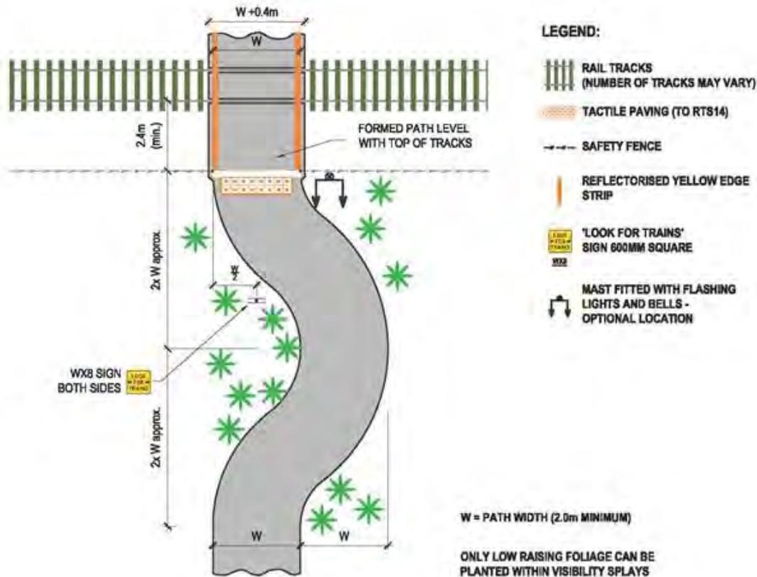
Figure 46: Layout plans for a curved deflection approach
