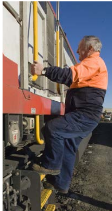
Driver climbing steep ladder to locomotive
