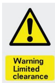
Figure 9.1 Example of limited clearance sign
